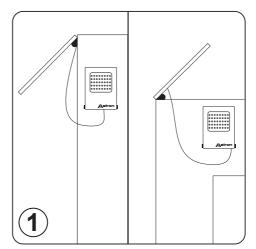
The Astron's solar panel can be mounted on either a vertical or horizontal surface as shown above. The Astron and solar panel are heavy so ensure your location is sturdy enough to take their weight.
