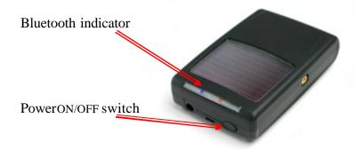
Push the power switch 1~2 seconds to Power on
