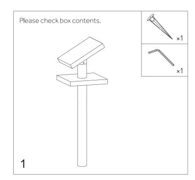
Make a hole by pushing the stake into the ground until the circular flange is just above ground level.
