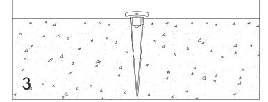
Raise the stake slightly and screw the light onto it. Now gently push the light back down into position.
