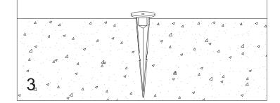
Raise the stake slightly and screw the light onto it. Now gently push the light back down into position.
