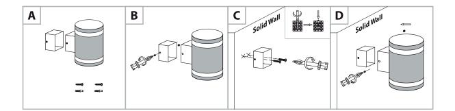
Choose a location with maximum sun exposure. Drill holes matching the pattern on the mounting plate as a guide, and install the plastic dowels. Attach the mounting plate using the screws provided. Secure the mounting plate onto the wall with the screws. Place the lighting fitting into the mounting plate and secure with the remaining screws provided.
